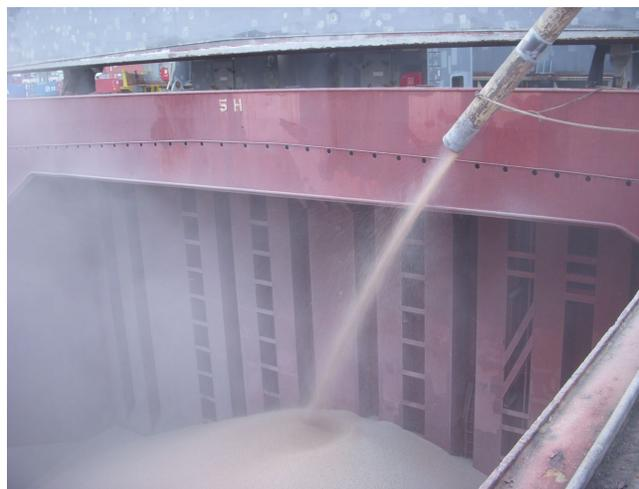
Figure 19 – Marine Spout Ship Loader
