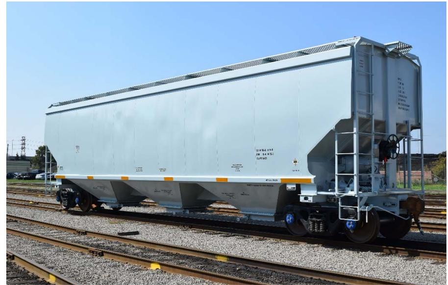
One of the new 5,431 cubic-foot hopper cars being produced by National Steel Car Limited at the company's facility in Hamilton, Ontario. With deliveries and committed orders for some 3,000 units, these cars are quickly becoming the successor to the cylindrical hopper cars that have been the backbone of the GHTS since the early 1980s. (Image courtesy of National Steel Car)
